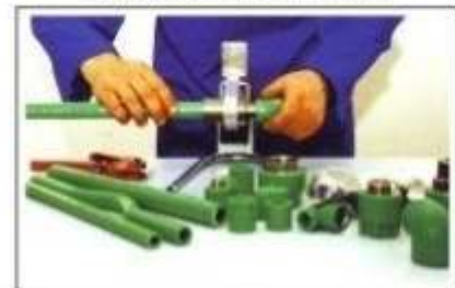
Fig. 2 Heat Pipe and fitting at same time
